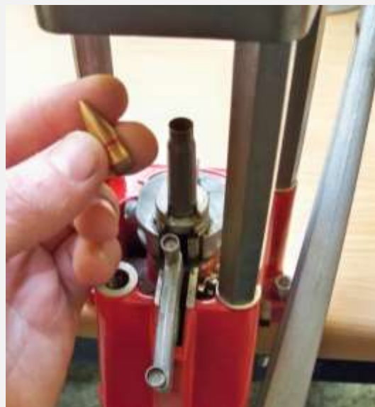
Loading a 7.62 x 39 round for the AK47 before firing in the lab ballistic range
