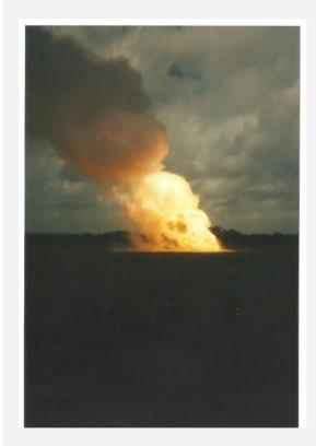
The deflagration of a substantial quantity of artillery propellent. Not a detonation but still highly destructive
